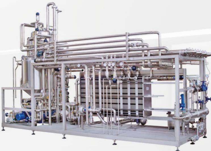
Ideal for processing low consistency products with a reduced fibre content, such as clear fruit juices and its concentrates, plate sterilizers are also used for fruit juices and isotonic drinks.
