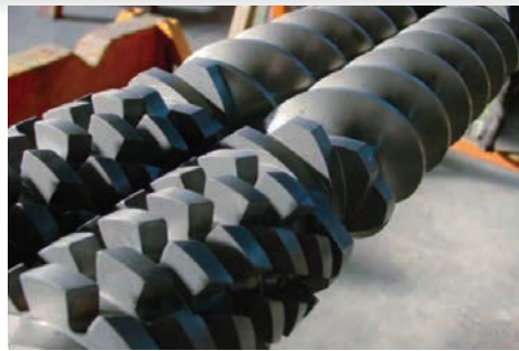
Extruders Screw designed and manufactured in UNION's factory.
