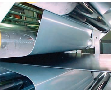
UNION extrusion line for composite panel. PE sheet coupling, type B-A-B, with aluminum foils.
