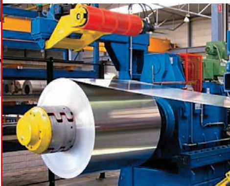
UNION extrusion line for composite panel. PE sheet coupling, type B-A-B, with aluminum foils.
