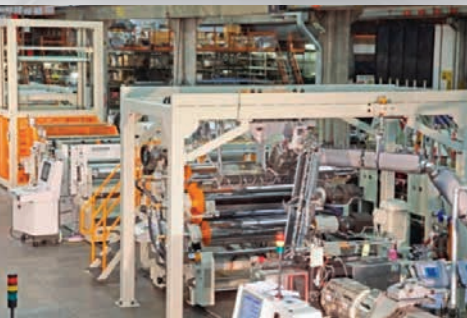
Assembly stage and testing of the extrusion lines.
