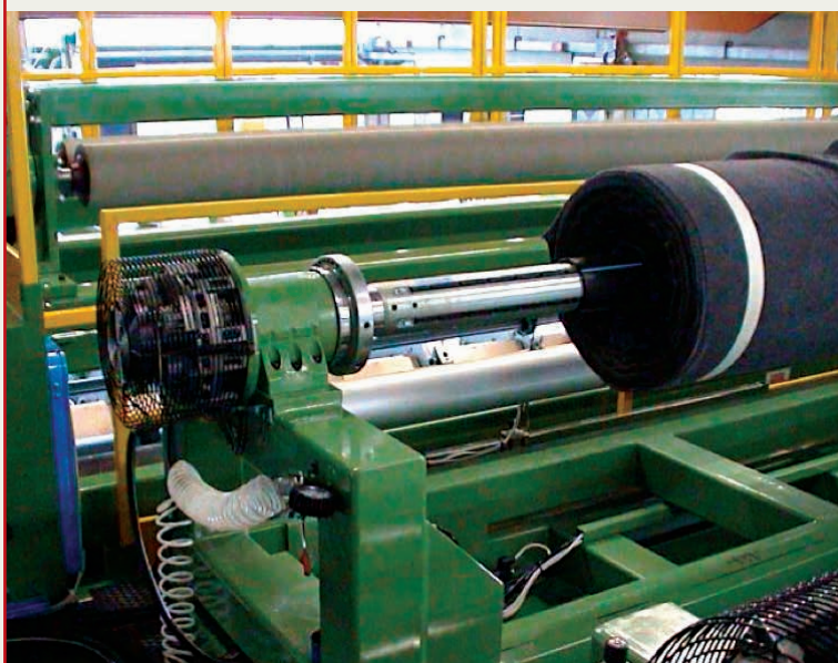
Coupling system with non woven material in polypropylene.
